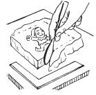
**Step 7:** Let the plaster soak for 3-5 minutes, then mix with your drill mixer. Mix for about 1½ minutes, then pour over boxed pattern. Plaster should cover at least 1 inch over the highest point on the Model.
