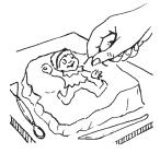
Step 6: READY FOR CASTING. For the size of the object shown in these drawings and the apparent bulk of parting line around the model, we will use the following proportions: With your 1 gallon plastic jar, weigh out 11/2 lbs. of No.1 Pottery Plaster; add plaster to 1 lb. of water. Always add plaster to the water, never water to plaster.
