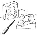
Step 15: At this time, check each half of the mold for any under-cuts that can be cut back. Let your mold dry out for 4 or 5 days depending on your weather conditions. NOW YOU HAVE A MOLD.
