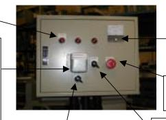
The voltage gauge Indicates the voltage input to the pug mill.
