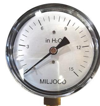
Figure 5 A close up of the Water Column Gauge on a Laguna Gas Kiln
